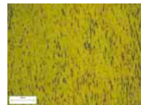
Large grain size associated with early fatigue failure - seen in a typical "forged 316L" femoral stem
