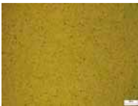
Grain size - seen at 100x magnification of the ENDOFIT femoral stem forged from high nitrogen stainless steel.
